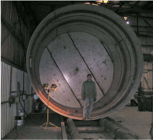
30,000 gallon 15' Diameter 316L Stainless Steel Storage Tank
